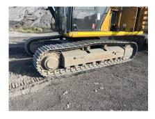
11.3 Inspect tracks for loose/missing bolts
