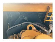
7.7 Inspect radiator and fan guard condition
