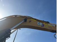
12.4 Inspect stick condition – cracks, missing clamps, damaged pipes, excessive movement, lubrication
