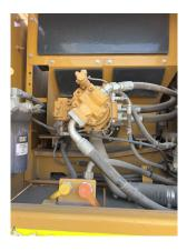
9.5 Check Pilot Accumulator operation as per OEM Maintenance Procedure -Test Boom Down Functionality with engine off
