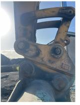
12.6 Inspect bucket condition – cracks, wear, damage, mounts
