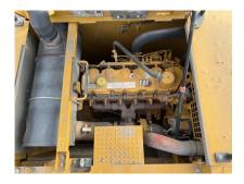
6.5 Inspect exhaust system for signs of leaks, loose bolts or missing clamps
