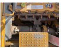
6.6 Inspect turbo for security and signs of leaks
